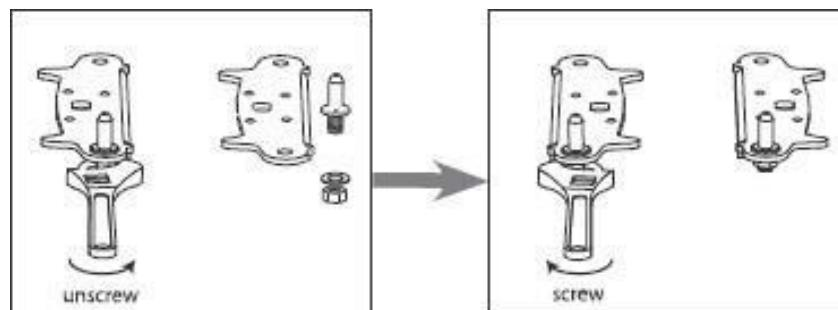
5. Refit the bracket fitting the bottom hinge pin. Replace both adjustable feet.
