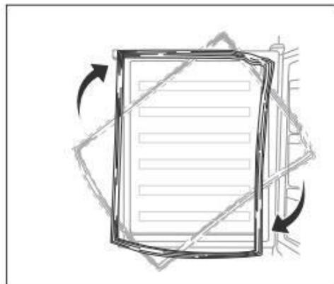
7. Place the door back on. Ensure the door is aligned horizontally and vertically so that the seals are closed on all sides before finally tightening the top hinge.
