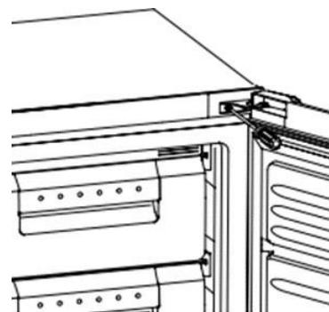
3. Remove the screws and bottom hinge. Then remove the adjustable feet from both sides.
