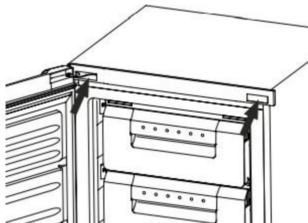
9. With the door closed, check that the door is aligned horizontally and vertically and that the seals are closed on all sides before finally tightening the bottom hinge. Re-adjust the levelling feet as needed.
