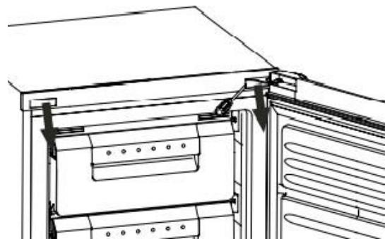
2. Remove the 2 screws, then remove the upper hinge that holds the door in place. Lift the door and place it on a padded surface to prevent it from scratching.
