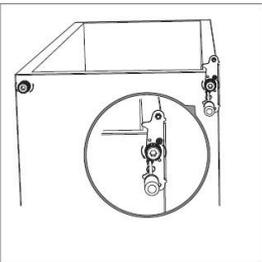
5. Unscrew and remove the bottom hinge pin, turn the bracket over and replace it.
