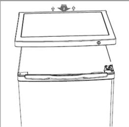
3. Unscrew top hinge, then remove door, and place it on a soft pad to avoid scratch.
