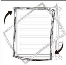
8. Place the door back on. Ensure the door is aligned horizontally and vertically, so that the seals are closed on all sides before finally tightening the top hinge.
