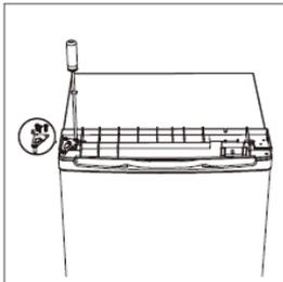
9. Put the top cover and fix it with 2 screws on the back..
