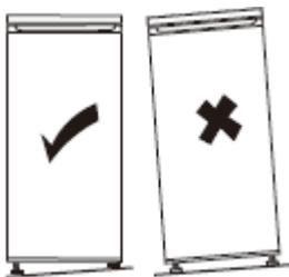
If the appliance is not level, the doors will not be correctly aligned and compartment sealing will not be ensured.
