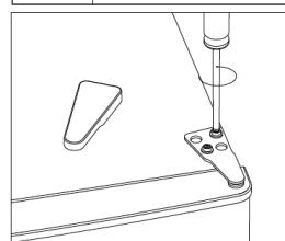
3. Remove the hole cover with a flat screw driver.
