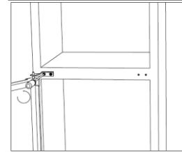
13. Install the upper door with the upper hinge.
