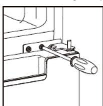
4. Laying down the refrigerator, take out the adjusting feet as below, then take off the lower hinge by cross screwdriver.
