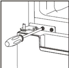
8. Place the upper door back on. Ensure the door is aligned horizontally and vertically so that the seal are closed on all sides before finally tightening the top hinge. Then inert the top hinge and screw it to the top of unit and then fix hinge cover (in accessory bag) by screw.
