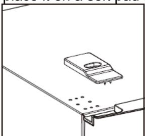
3. Remove the top left screw cover. Take off the upper door, take out the screw from the middle hinge by cross screwdriver, then take off the lower door.
