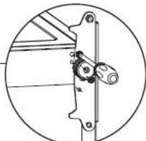
5. Adjusting the hinge core position of the lower hinge and upper hinge to opposite position
