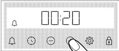
» After setting the alarm time, the
