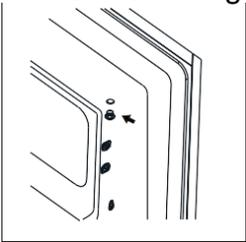
7. Rotate freezer door and place hinge side at left side and then fix the door by holder.
