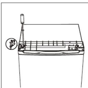
12. Put the top cover and fix it with \$ screws on the back
