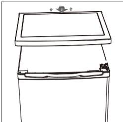
3. Unscrew top hinge and then remove door and place it on a soft pad to avoid scratch.
