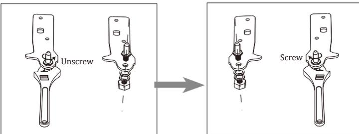
10. Refit the bracket fitting the bottom hinge pin. Replace both adjustable feet.
