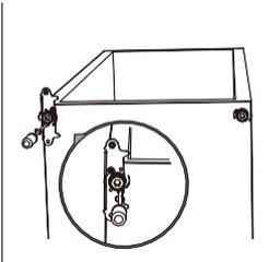
11. Place the door back on. Ensure the door is aligned horizontally and vertically, so that the seals are closed on all sides before finally tightening the top hinge.
