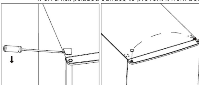
4. Unscrew the middle hinge. Then lift the lower door and place it on a flat padded surface to prevent it from being scratched.
