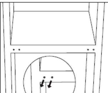
6. Tilt the appliance back, then unscrew the lower hinge. Then remove the adjustable feet from both sides.
