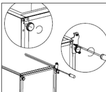
7. Unscrew the mounting plate with the lower hinge pin and refit it.
