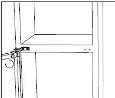
11. Refit the upper door. Make sure that the door is horizontally and vertically aligned so that the seals are tight on all sides before tightening down the upper hinge. Then insert the hinge and screw it onto the top of the appliance.
