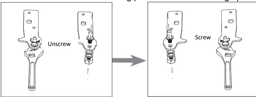
8. Transfer the lower hinge from left to right. Refit the two adjustable feet.
