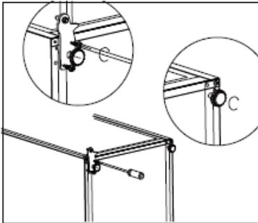
9. Bring the appliance upright again and refit the door onto the lower hinge. Make sure that the hinge is correctly inserted into the door. Then, transfer the lower door hole covers from left to right.
