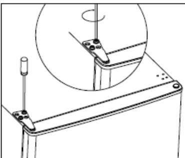
12. Reclip the hinge cover and refit the hole cover onto the top of the appliance.
