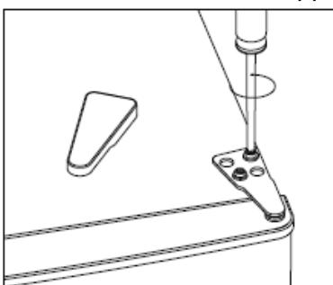
3. Remove the hole cover and transfer it from left to right, then remove the upper door and place it on a flat padded surface to prevent it from being scratched.
