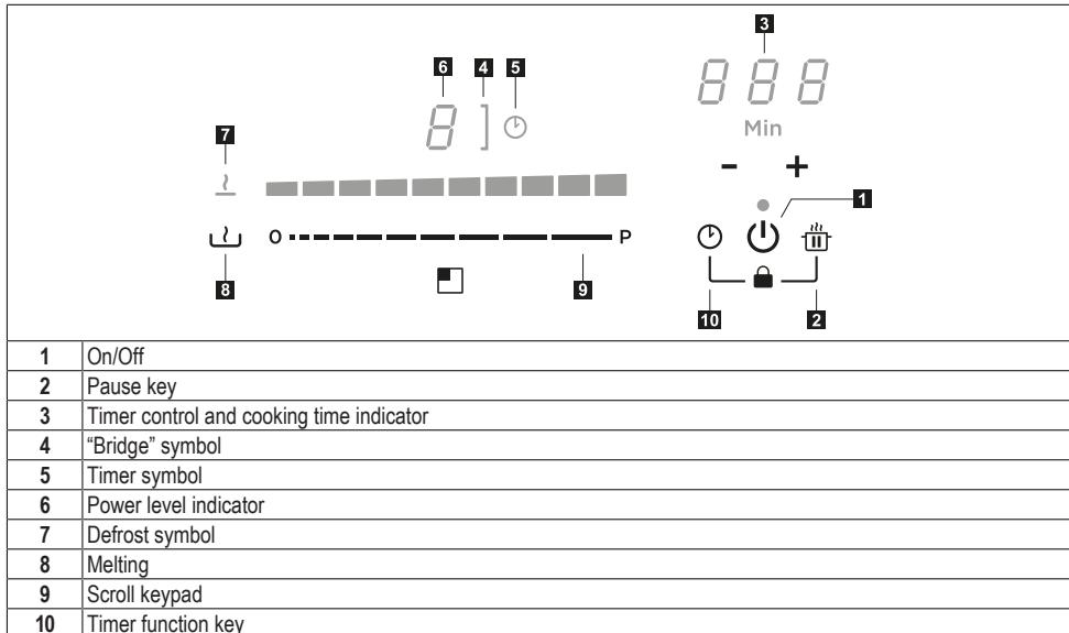
The cooking zones can be activated by pressing the reference digit **8**. The digit becomes brighter to confirm the operation.
