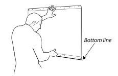
Mark the position of the fixing holes on the wall.
