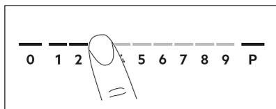
1. Press the desired heat setting on the control bar. You can also move your finger along the control bar to set or change the heat setting for a cooking zone.
