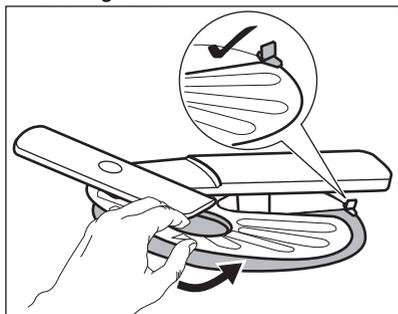
7. Reassemble the filters (B) and (C).
