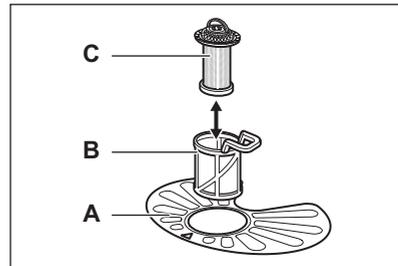
1. Turn the filter (B) counterclockwise and remove it.
