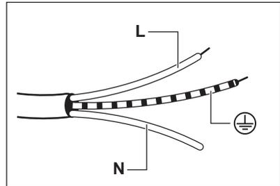
1. Connect the green and yellow (earth) wire to the terminal which is marked with the letter 'E', or the earth symbol
