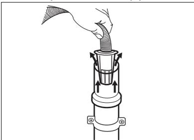
5. **Without the plastic hose guide, to a sink spigot** - Put the drain hose in the spigot and tighten it with a clamp. Refer to the illustration.
