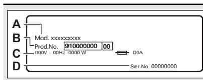
The rating plate reports the model name (A), product number (B), electrical ratings (C) and serial number (D).
